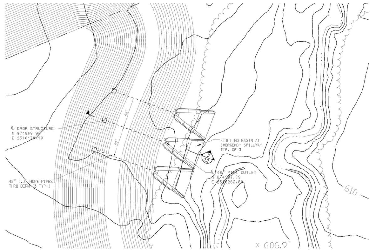
1 STILLING BASIN PLAN AT EMERGENCY SPILLWAY
