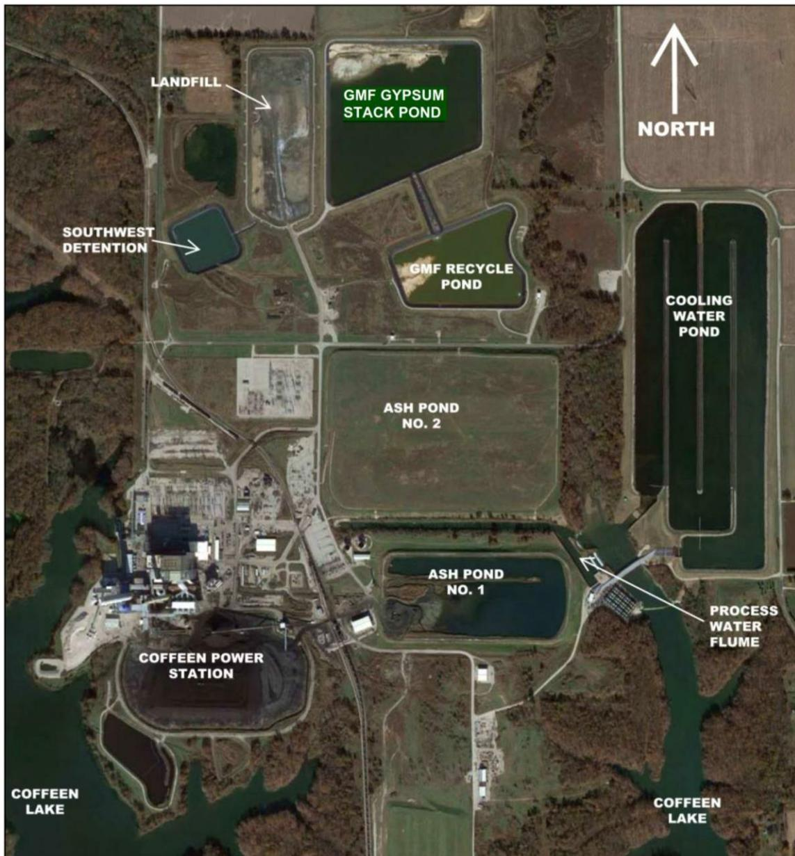
Figure 2 – Site Plan (adapted from AECOM, 2016)
